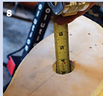
7. Continue drilling straight into the foam to a depth of 4 inches. 8. The length of the TPS-100 receiver is 4 inches.
