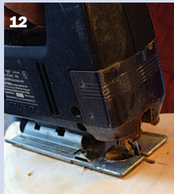
12. A jigsaw is used to cut out the drawn wing lines. 13. The receiver hole is ready to insert the receiver.
