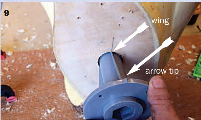
9. Push the receiver into the hole until the three side-wings fit tightly. The parts have a pre-established alignment system. Note that the arrow tip located on the top of the receiver is in alignment with the wing that you need to also align with the line drawn on the plywood.
