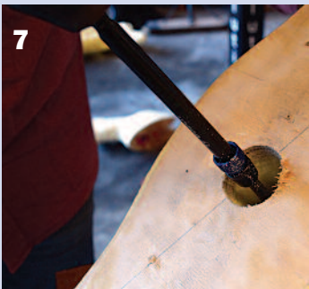
7. Continue drilling straight into the foam to a depth of 4 inches. 8. The length of the TPS-100 receiver is 4 inches.
